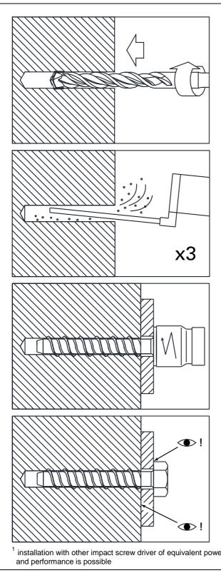
Drill hole with rotary percussive machine. Drill to a required depth.
